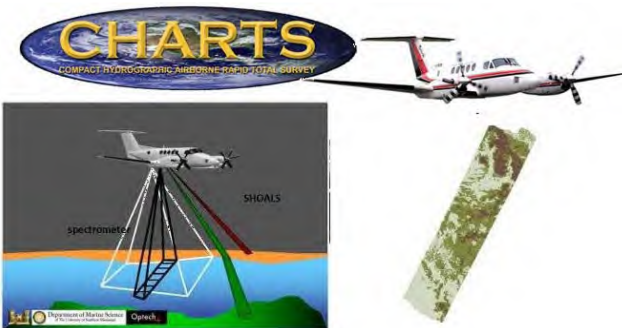
Figure 6-14. USACE GPS-controlled CHARTS hydrographic surveying system (JALBTCX)
