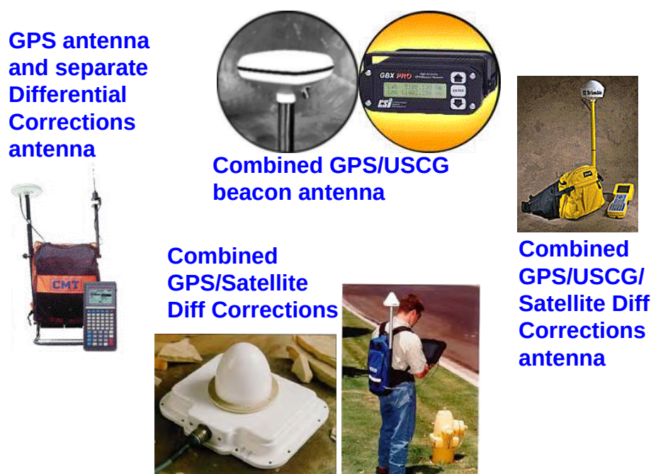
Figure 7-3. Common data links for code and RTK GPS receivers
