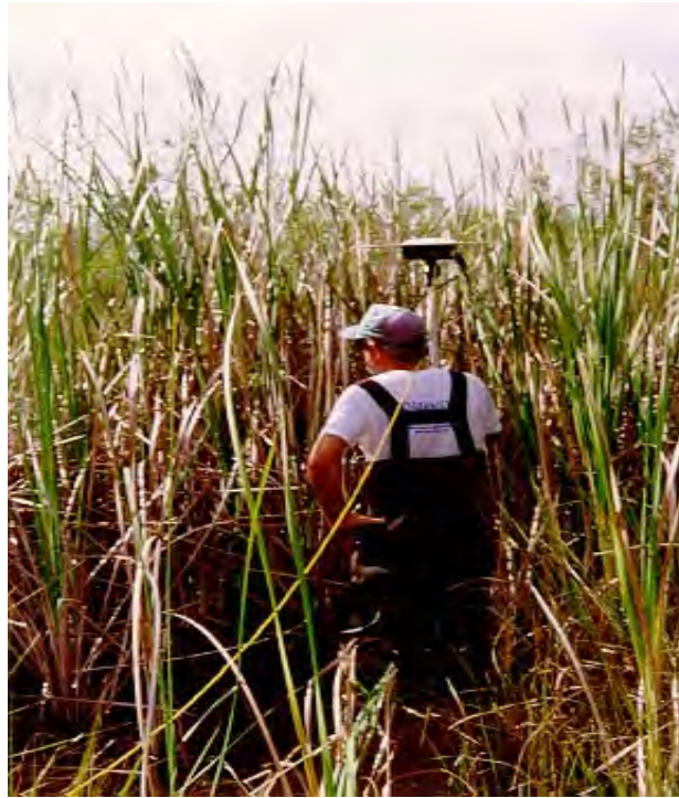
Figure 6-3. GPS real-time kinematic topographic surveys using backpack and range pole antenna mount
